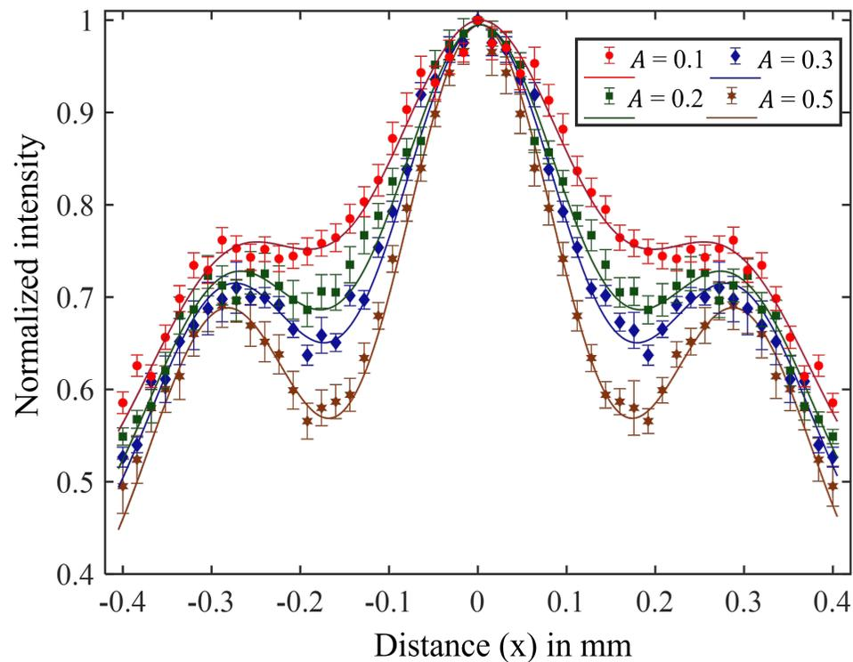
Double-slit interference using signal beam of single photons
