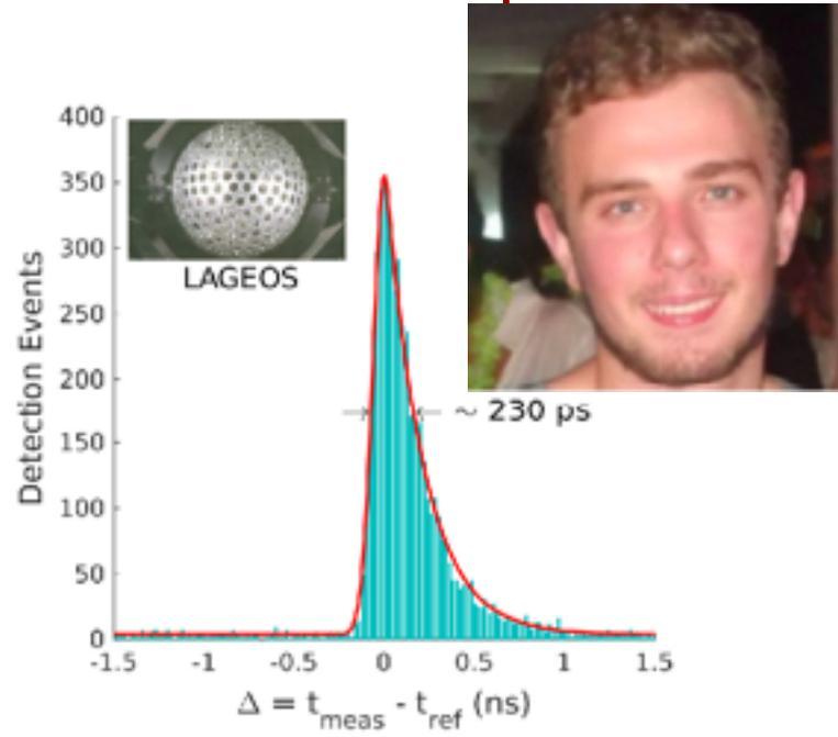
The 100-MHz pulse train is detected after a 50:50 BS to separate the outgoing and incoming beams and 3 nm spectral filter a silicon single photon avalanche detector SPAD (Micro-Photon-Devices Srl) with  $\approx 50\%$  quantum efficiency,  $\approx 400$  Hz dark count rate and 40 ps of jitter.
