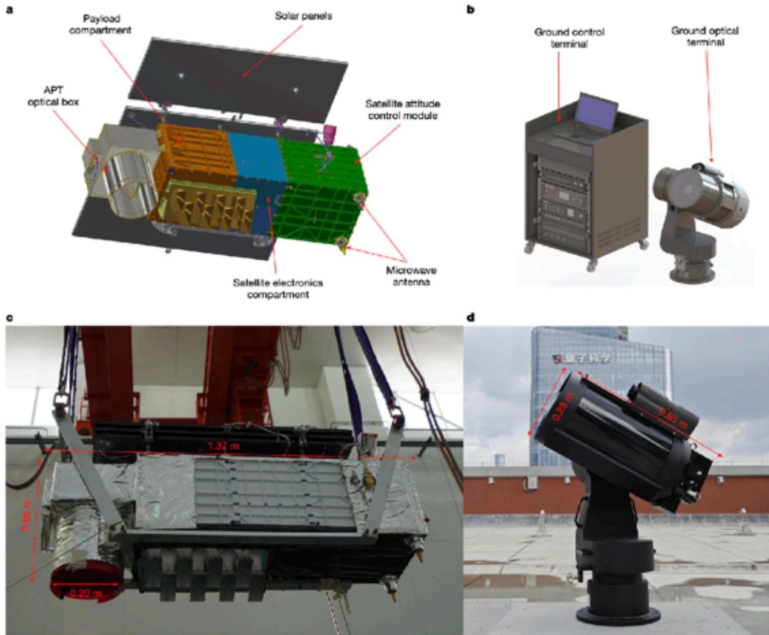
**Fig. 3 | The microsatellite and the portable OGS.** **a.** The satellite consists of an APT optical box, payload compartment, satellite electronics compartment, satellite attitude control module, microwave antenna and solar panels. **b.** The OGS consists of a control terminal and an optical terminal. **c.** Photo of the microsatellite before being assembled into the rocket. The satellite launch
