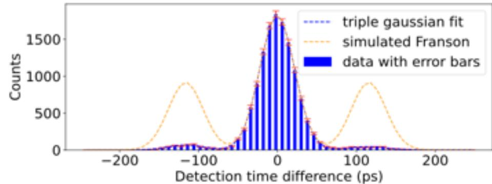
Histogram of detection time differences for arrivals at detectors  $D_{A_{+1}}$  and  $D_{B_{+1}}$  with bin-width of 8 ps.
