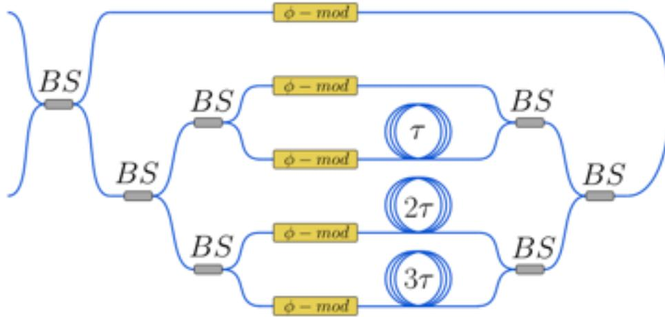
Scheme for the generation of four dimensional states **using two by two beamsplitters** in a series of two interferometers
