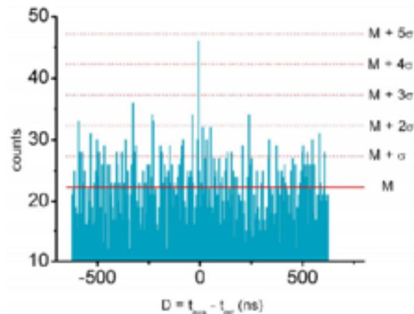
**Figure 3.** Histogram of the differences  $D$  between expected and observed detections for Ajsai satellite. The peak of the histogram is centered at  $D = t_{exp} - t_{ret} = 0$  ns, as expected, and is larger than the mean value of the background counts by 4.5 standard deviations. The bin size is  $\Delta t = 5$  ns.
